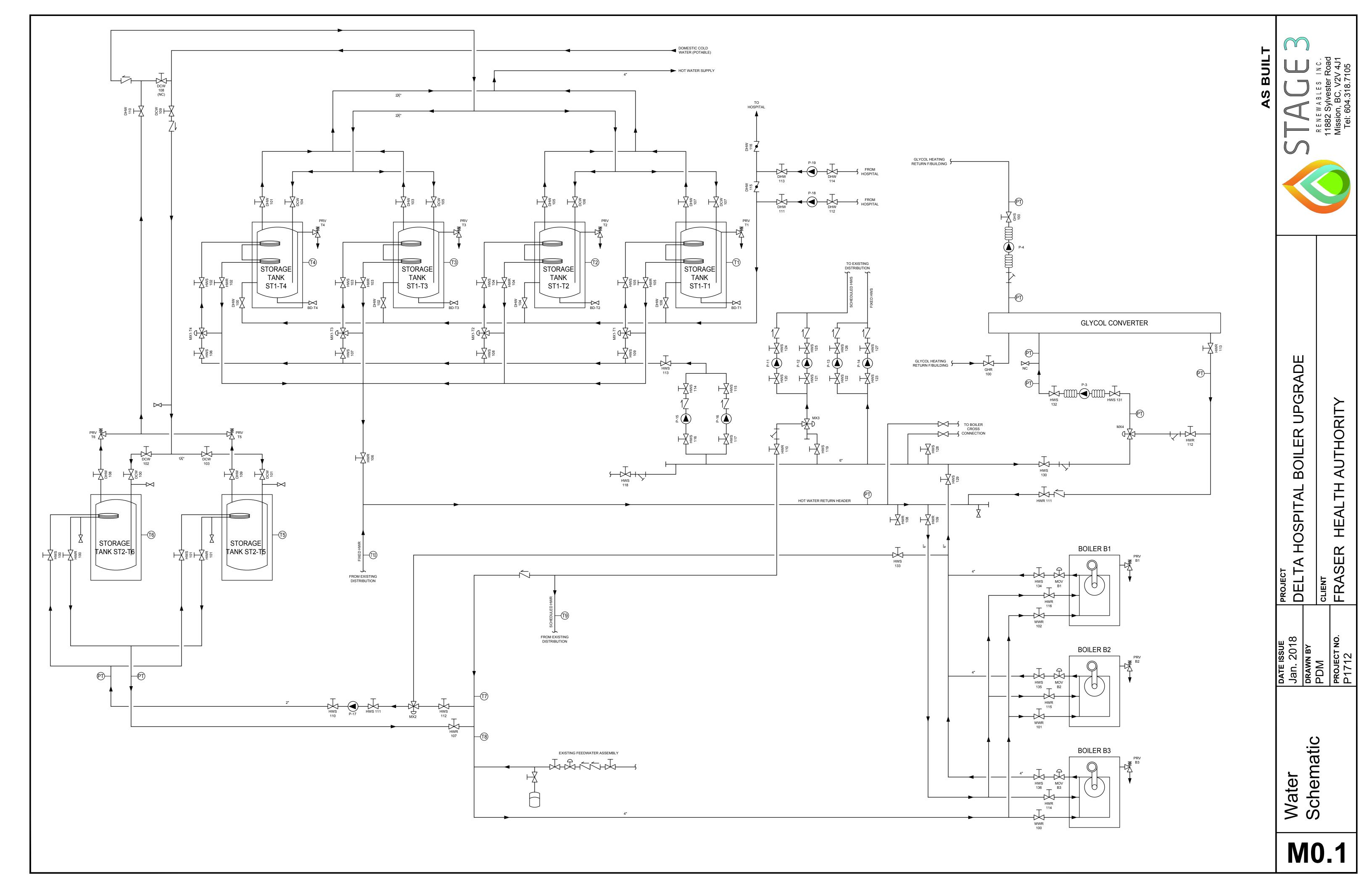
NOTE: COMPONENT UNIONS AND ISOLATION VALVES NOT SHOWN CLARITY ACTUATOR END SWITCH ON EXISTING PREHEAT COILS TO START PUMP ON FULL CLOSE OF ENERGY VALVE.
